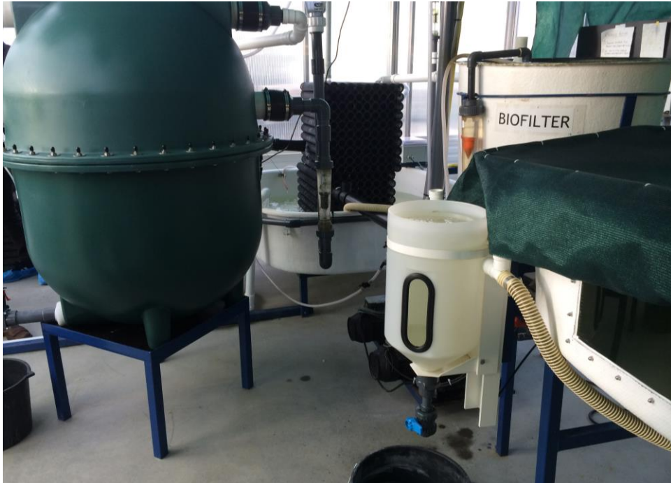
Figure 3.3 Bead filter, trickling filter, moving bed bioreactor and swirl separator
