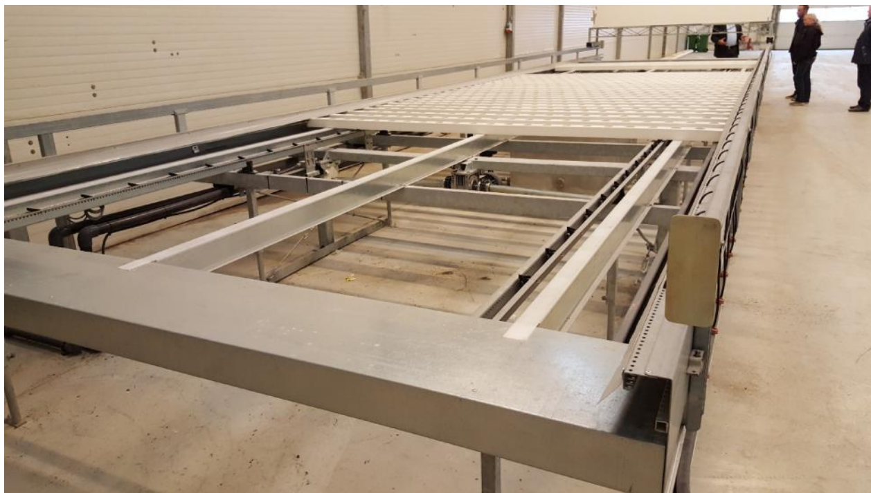
Picture 3. The moving gutter system using NFT piping illustrating how an industrial design does not make it feasible to have fish tanks underneath, or if redesigned, would not make a daily monitoring optimal at all.
