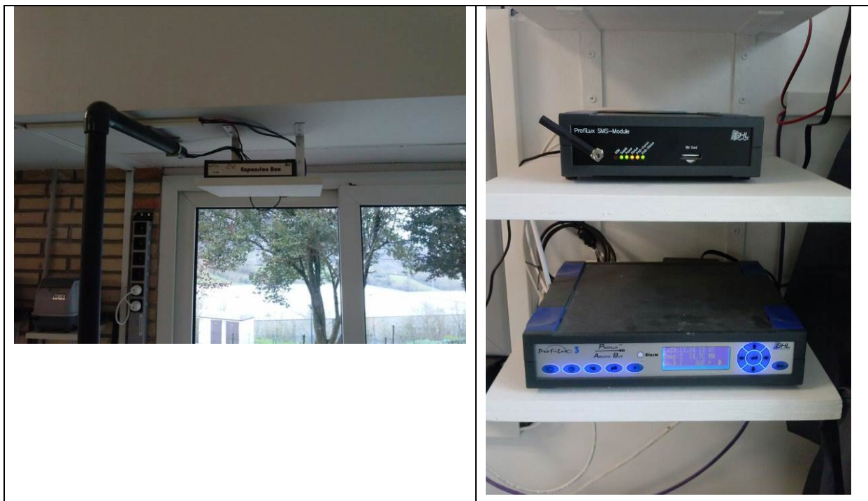
Figure 4. The Profilux expansion box (left) and the Profilux SMS, above and Profilux 3, below (right).
