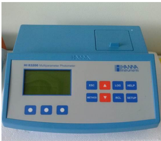
Figure 5. Spectrophotometer from Hanna Instruments.
